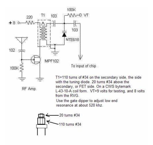
*10/06/06* I like this detector for the LM3820 better than the FET detector I had in the schematic.
