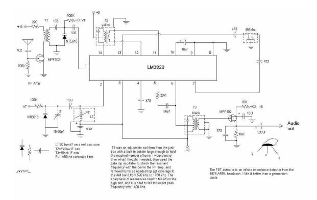
**01/12/07** This is the RF amp I use for the short wave converter, placed after the AM BCB filter, going to the NE602 mixer. I found that the MPF102 works about 100% better than the J309, or J310 FETs. Using relays, in shortwave mode I switch the AM tuner to a fixed tuning voltage that comes from the 8 volt regulator through a trim pot, setting the tuning for roughly 1MHZ (1455KHZ l.o.) then tune the converter using the VT signal from the RVG using a red LED as a tuning capacitor.
