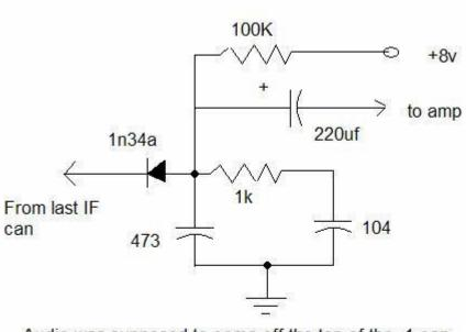
Audio was supposed to come off the top of the .1 cap, but I liked the level at the anode of the diode better. to take the audio from the oterh end of the 1oK resistor, reduce the size of the .1 capacitor to maybe .003 uf.
